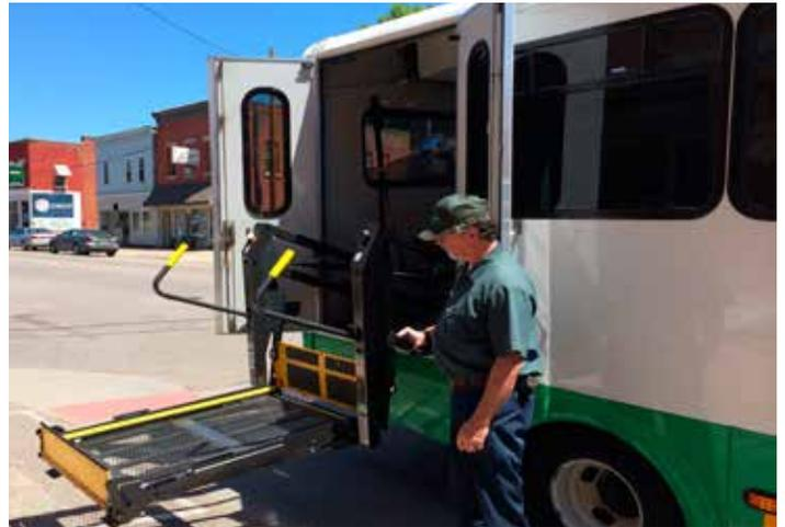
A bus driver showcases one of the lifts that are installed on many of the Jule busses
